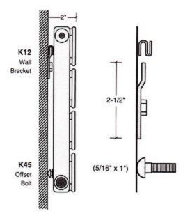
R clip - Mount to the grille back on the R Radiator at the K12 Positions
