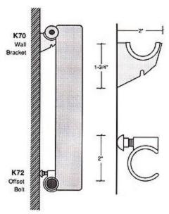
**K70** Wall Bracket - Support Bracket used at the top header of the Radiator
