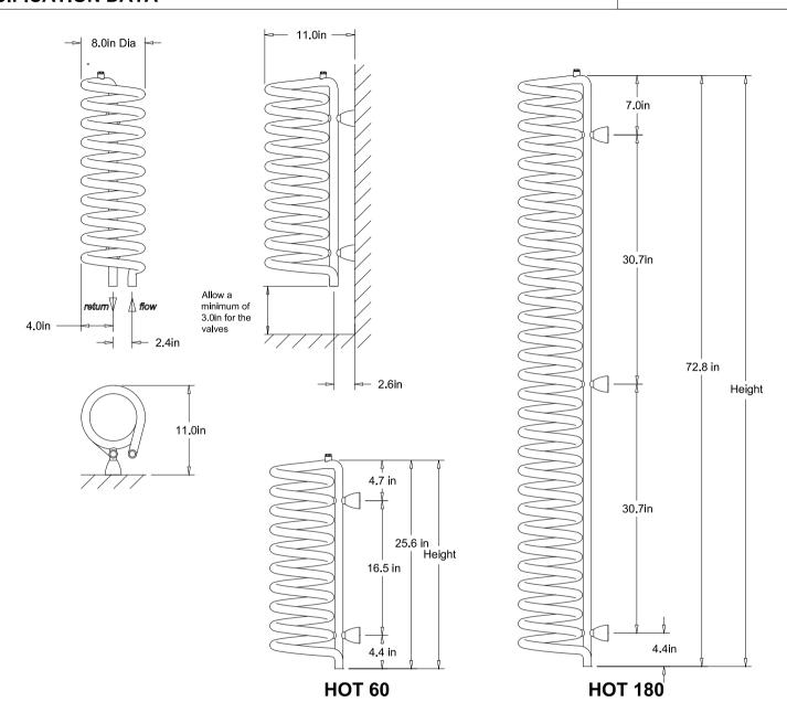
Test pressure: 174 P.S.I. 100 P.S.I. 200 °F Max working pressure: Max working temperature:
